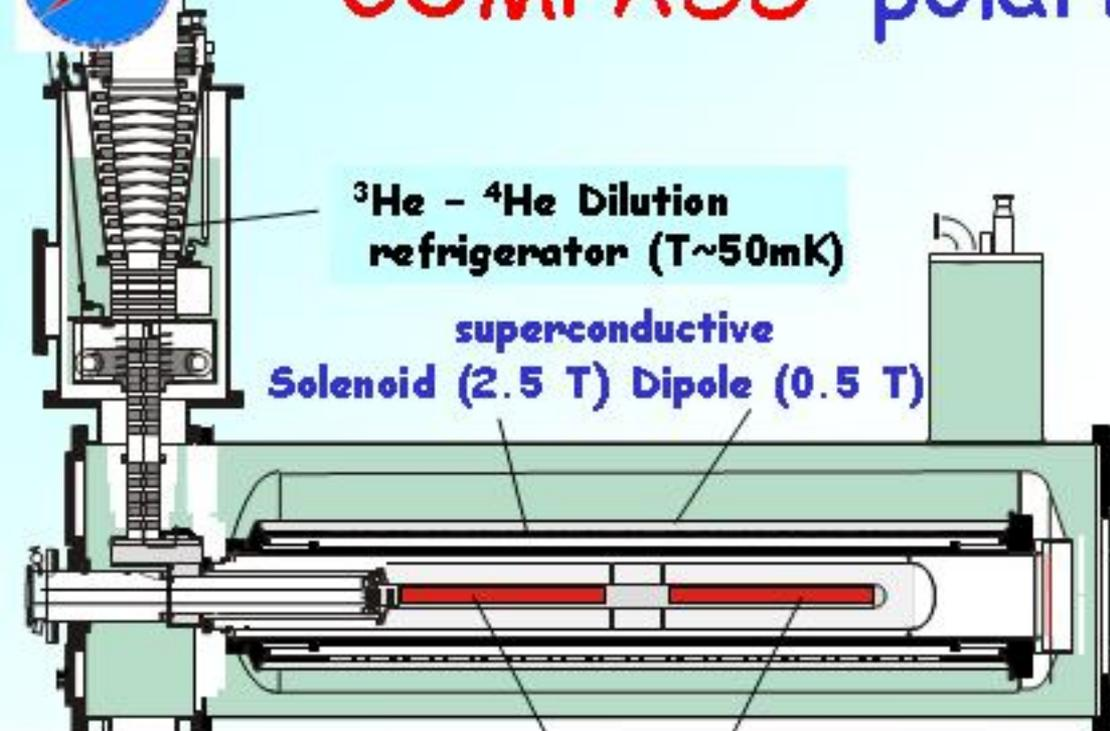
$^3\text{He} - ^4\text{He}$  Dilution refrigerator ( $T \sim 50\text{mK}$ )
